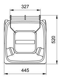
Mobile Garbage Bins MGB 80 Litre Sizes, Measures, Dimensions: Hight 939 mm; Width 445 mm; Depth 520 mm
