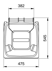
Mobile Waste Containers MGB 120 Litre Sizes, Measures, Dimensions: Hight 930 mm; Width 475 mm; Depth 545 mm
