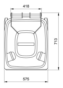
Mobile Waste Containers MGB 240 Litre Sizes, Measures, Dimensions: Hight 1063 mm; Width 575 mm; Depth 713 mm
