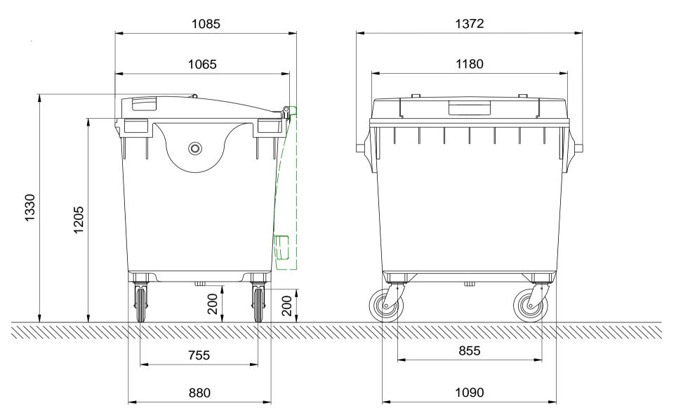
Mobile Waste Containers MGB 1100 Litre Flat Lid - Lid in Lid Sizes and Measures: Hight 1330 mm Width 1372 mm Depth 1065 mm
