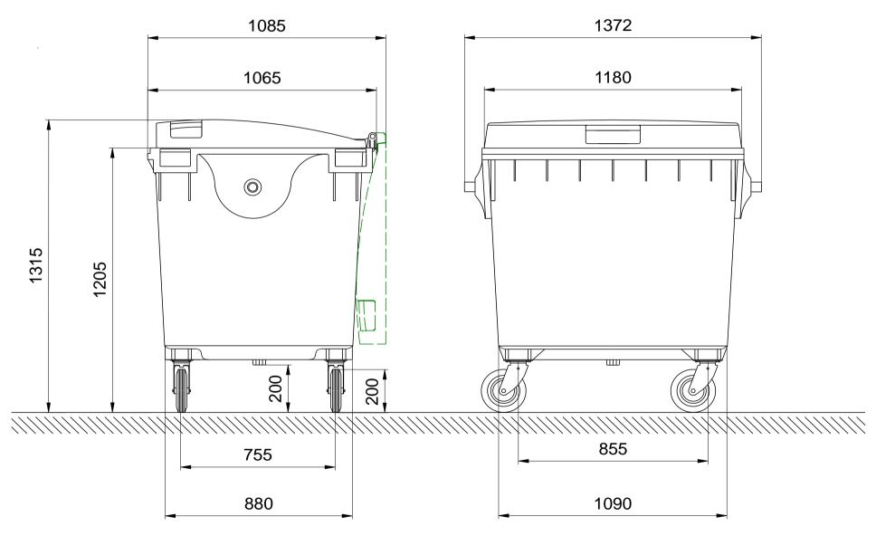
Mobile Waste Containers MGB 1100 Liter Flat Lid Sizes and Measures: Hight 1315 mm<sup>-</sup> Width 1372 mm<sup>-</sup> Depth 1065 mm
